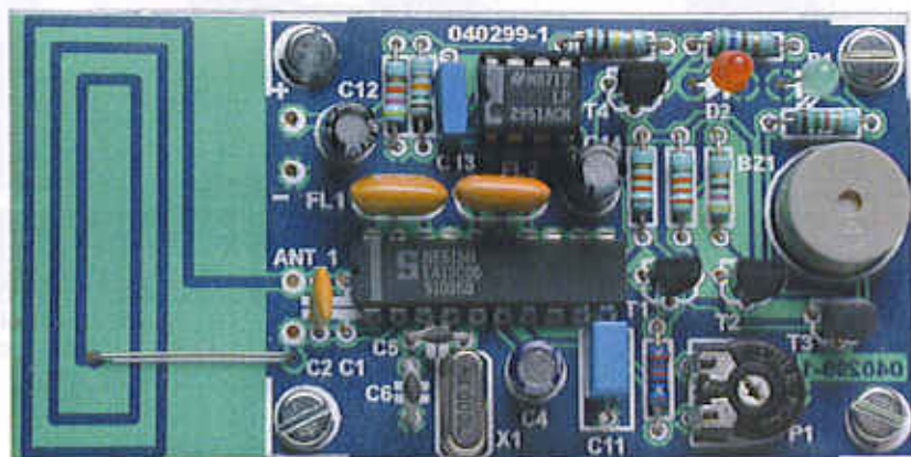
Figure 5. Top side of the board with all the parts fitted. Note the wire link connecting the stripline antenna to C2/C1.
