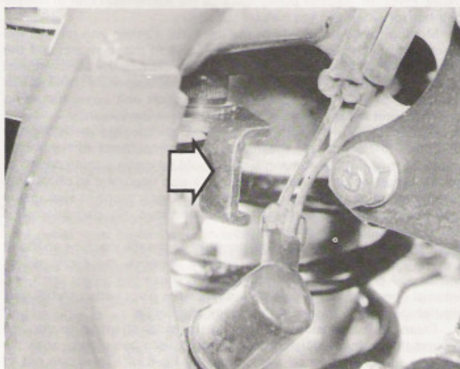
10.8a Tension belt by pressing lever (arrowed) ...
