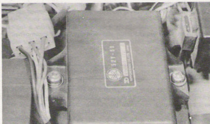
7.1 Ignition coil is bolted to frame below the fuel tank
