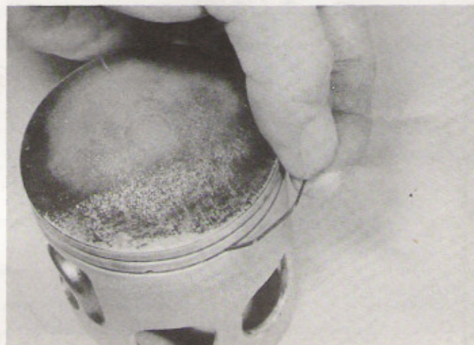
18.5a Note how ring ends locate over peg in ring grooves
